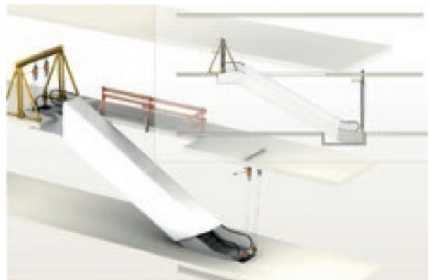
Figure 8.5 Installation using a lifting frame
